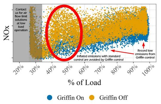
One year of closed-loop operation on a 500 MW coal-fired unit comparing NOx emissions while Griffin COS is active and inactive. The Griffin COS realized an average NOx improvement of more than 20%.
